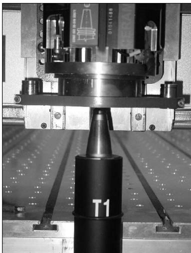
**Note:** On 250mm axis machines you will have to jog the head down so the air cylinder will reach the spindle.
