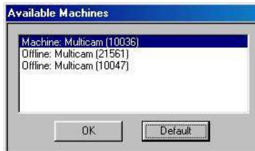
If you are presented with the dialogue box shown below this means that whilst ToolPath is able to communicate with your machine, there is no operating system on the machine and it must be downloaded to it
