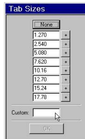
Tabs are placed evenly around the perimeter of the shape commencing from the Start Point of the shape. If the tab placement does not seem correct then you can re-position the tabs by moving the Start Point of the shape. Refer to page [51](#) for more information about Start Points.
