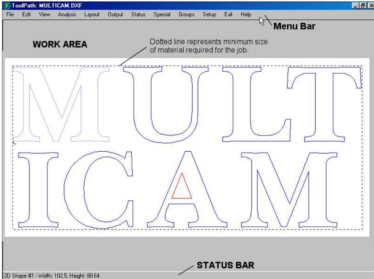
The Status Bar is at the bottom of the screen and displays information about your job (such as shape size, overall size, number of shapes etc) it will also display a progress bar when transmitting jobs to your machine or importing files.
