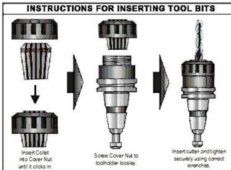
**Note: To ensure trouble free operation, always insert the collet into the collet nut until it clicks in, and tighten loosely onto spindle prior to inserting tool bit. If manually changing tools in a quick tool change motor ensure that the tool holder is correctly engaged in the motor. Do this by firmly grasping the nut on the tool holder and pulling in a downward and sideways movement and checking for looseness. If you are able to “wobble” the tool holder it is not correctly engaged.**
