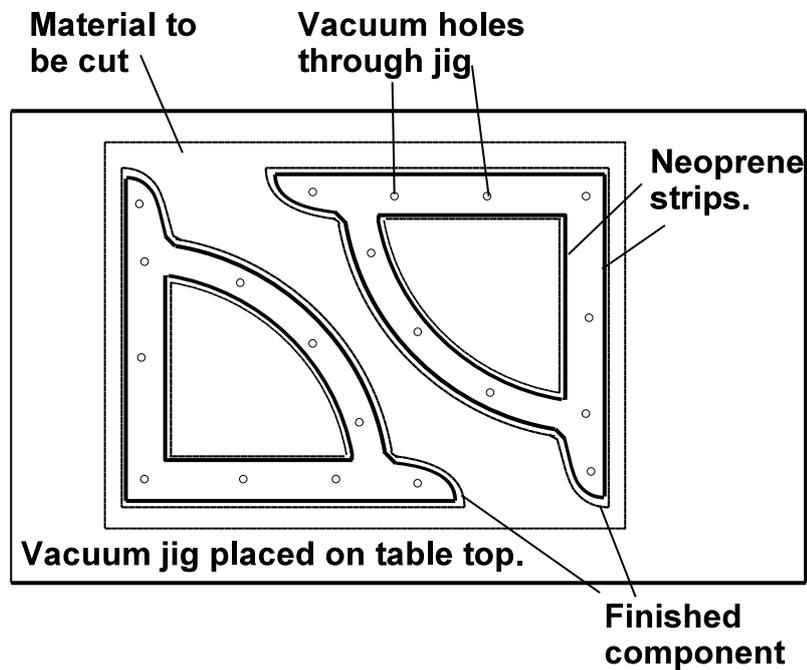
Another advantage of this type of arrangement is that it allows you to use small and irregular shaped materials from which to cut your components. This is useful where the routing operation may come after some other machining process such as sawing.
