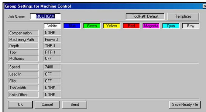
Functions that affect the way the job is cut can all be set in the **Output** dialogue box by clicking on the value on any one of the group fields (i.e Compensation, Machining Path, Depth etc..)
