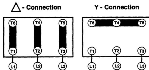
3.5HP Perske spindles are wired in their terminal block in a *DELTA* ( $\Delta$ ) pattern.
