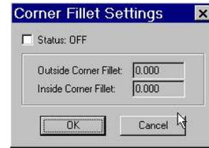
From the **Corner Fillet Settings** dialogue box check the Status check box and click on either **Outside Corner Fillet** or **Inside Corner Fillet**.
