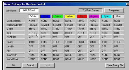
For example a 3mm spiral cutter may be associated with the White group which is always associated in your designs with cutting straight through your material, and a 90° Vee groove cutter may always be associated with the Blue group.
