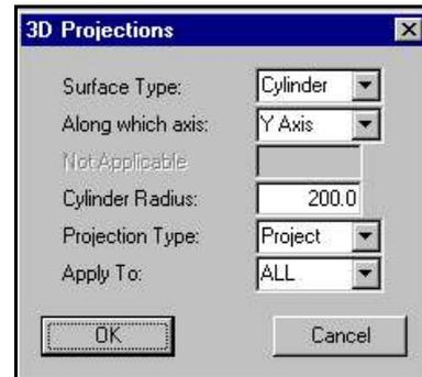
*Note: When engraving over a Cylindrical or Spherical surface you should use a ball nose cutter that will allow machining over a curved surface. Flat bottomed cutters will cause gauging in the bottom of your job.*
