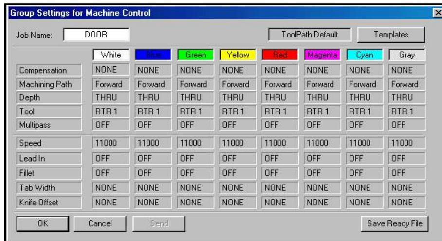
For each group you may set the Compensation, Machining Path (direction), Depth, Tool, Multipass, Speed, Lead In, Fillet, Tab Width or Knife Offset.
