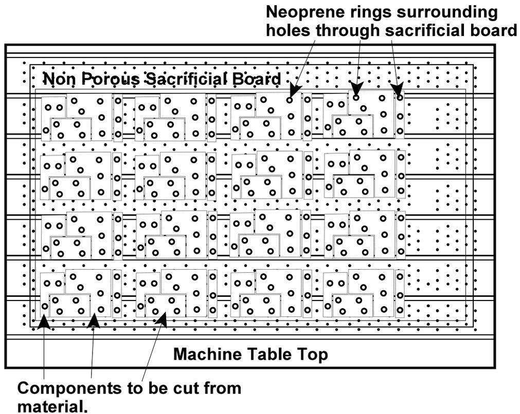
Use something non-porous such as plastic as your sacrificial sheet. Drill some holes in it then stick some neoprene tape or donuts around the holes. Place your process material on top of the neoprene tape.
