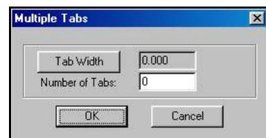
Tabs are useful if you are cutting lots of small shapes that threaten to pop out and jam the cutting head or get damaged by fouling the router bit once they are cut. It is also useful if you are cutting thick materials such as aluminium and perspex.
