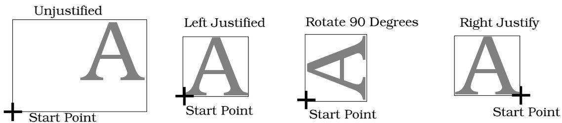
**Unjustified** This means that the starting position of the cutting head is the (0,0) co-ordinate of the job.
