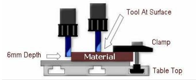
Here you can enter the depth at which the machine should cut the job. **THRU** indicates that the machine will cut right through the job to the bottom of your Function 4 setting. This is the setting mostly used for cutting out shapes. If you do not want to cut right through your material enter the depth to which you want the machine to cut and then click the **OK** button.
