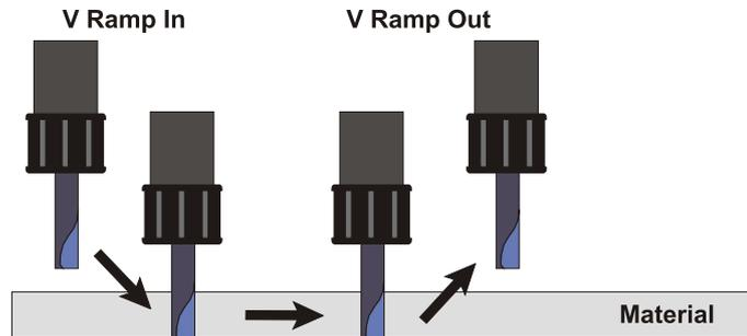
To enable V Ramping you must firstly enter a depth in the Lead In/Out Settings dialogue box, then check the V Ramp check box. The depth that you enter here will automatically be transferred to the depth setting in the Group Settings dialogue box. If there is already a depth set (other than THRU) in the dialogue box then you will notice that this depth is already placed in the Lead In/Out Settings dialogue box, so all you need to do check the V Ramp check box to enable the function.
