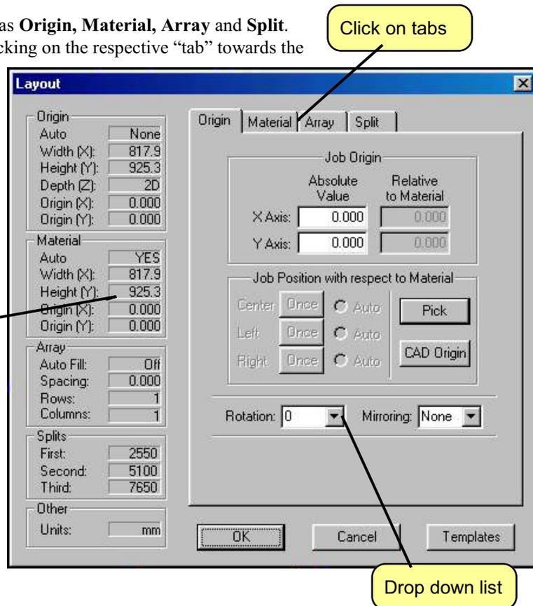
The job width and height are determined by the file that is imported. An important thing to remember is that the units of measurement are set in the **SETUP** menu. **ToolPath** defaults to MM. If you want to change this to CM or INCHES, refer to the section on **SETUP**. It is vital that the values that are exported from your design program are the same as those you are working with in **ToolPath**.
