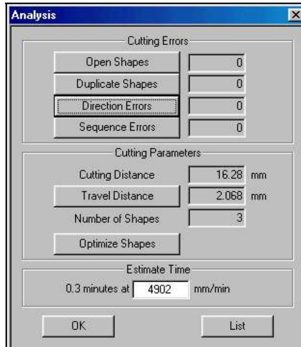
**ToolPath** will automatically correct direction, sequence and duplicate shape errors when you click the corresponding buttons in the dialogue box. You should always ensure that there are no direction or sequence errors in the job before transmitting the job to the machine.
