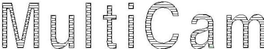
2D design after the tool path has been calculated showing the actual tool path within the lettering and hatching.
