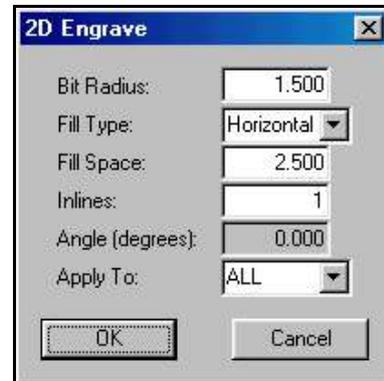
Once the engraving has complete you may accept the result by selecting **Enter**. If it is not satisfactory, select **Undo** and try a different bit size, fill space, or fill type, or a combination all three.
