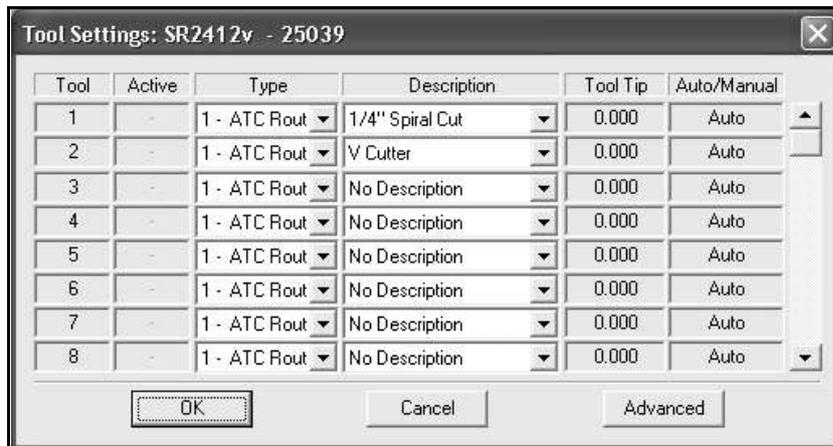
Selecting the Configure Tooling button on the bottom right corner of the Machine Info tab, you can set up the number and type of tools your machine is equipped with. These settings allow you to set a different tool for different groups in your job. You can configure up to 16 tools mapped at up to 4 physical tool positions. A physical tool position corresponds to an actual tool on your router table (i.e. Router, Drill, Automatic Tool Changer (ATC), etc).
