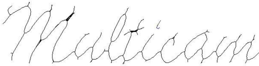
The resulting 3D tool path that has been generated. The tool path shown represents only the path the point of the 3D tool will travel.
