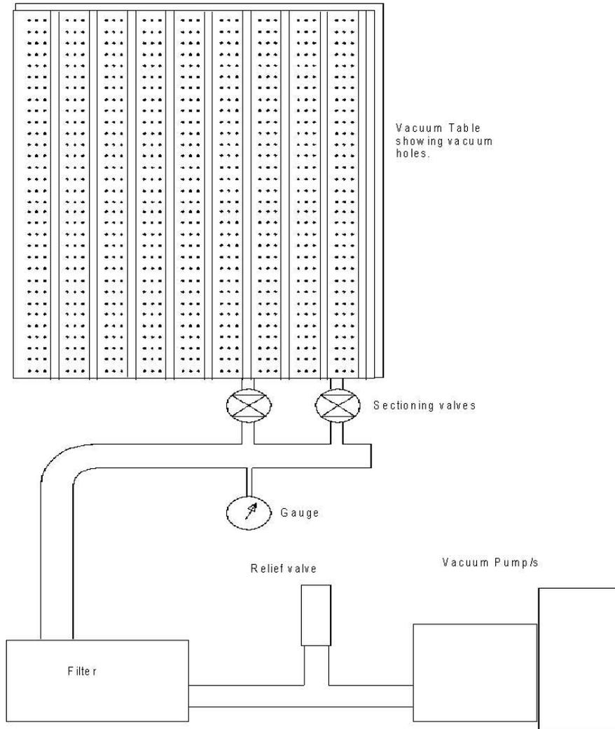
**Vacuum Table** The standard vacuum table has a series of holes machined in the top of the table through which air is drawn. The table is sectioned off according to the number of control valves giving active "zones" on the table.
