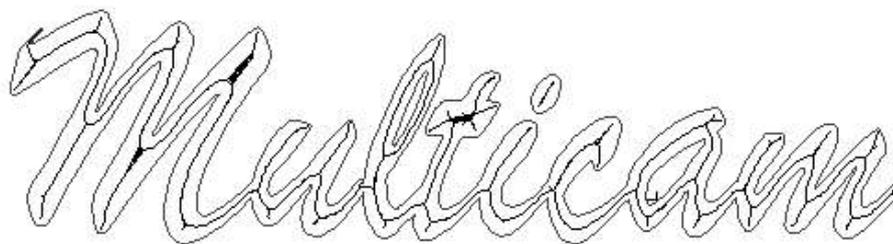
3D design after the tool path has been calculated showing the actual tool path within the lettering and some small areas of hatching.
