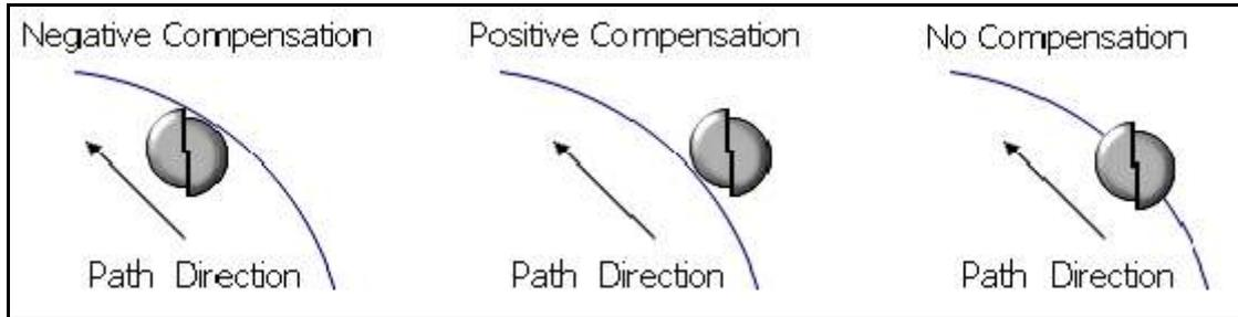
The radius (or half the diameter) of the bit is used as the compensation amount. Select the appropriate compensation by clicking on either the + button next to the required value for positive compensation or the - button for negative compensation. You can also enter a custom compensation value by entering the value in the Custom box and clicking the **OK** button
