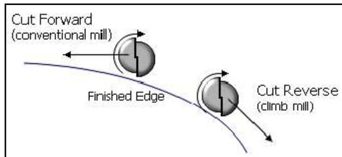
A **Forward** machine path is referred to as “Conventional Milling” in the industry. This means that outside shapes cut Counter-Clockwise and inside shapes cut Clockwise. This is the preferred path direction when cutting wood and most plastics.
