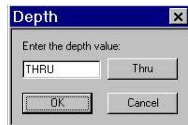
**NOTE:** For safety it is always preferable to enter the thickness of your material (plus a small cut through allowance of say 0.2mm) in the depth setting field. This will prevent you from plunging in to your machine table top in case you accidentally incorrectly set your Function 4 setting.
